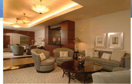
Park Laurel Lobby - Each chandelier was illuminated with five 100-watt lamps which generated so much heat extra cooling vents were designed into the soffits. With only three 13-watt lamps in each chandelier, Park Laurel reduced energy consumption for lighting and cooling, while maintaining lumen output that showcases the beauty of the custom onyx fixtures.
